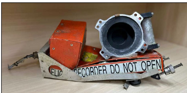
Figura 30 - Cockpit Voice Recorder instalado na aeronave PS-VPB.
